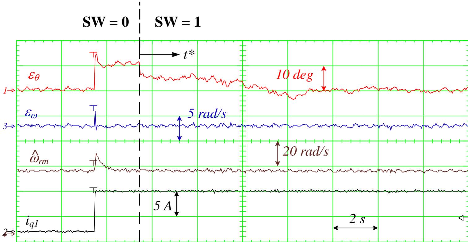
Activation of the MVPT algorithm on the estimated rotor position at the instant  $t^*$
