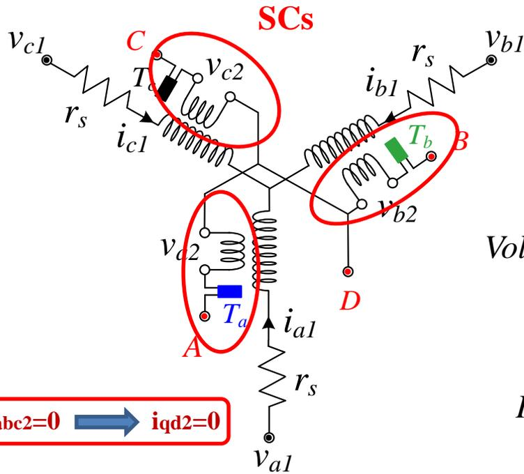
Equivalent circuit of the electrical machine including search coils
