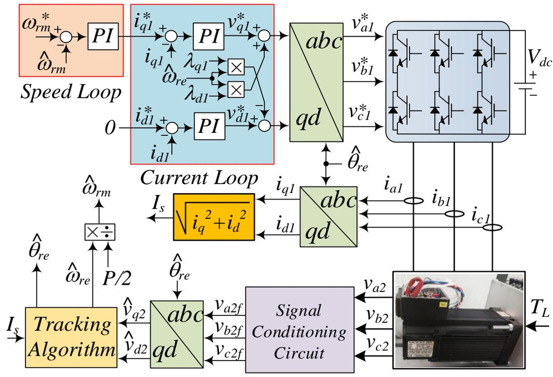
Block diagram of the sensorless motor drive
