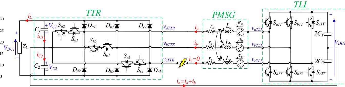
1. PMSG Model during open-phase fault
