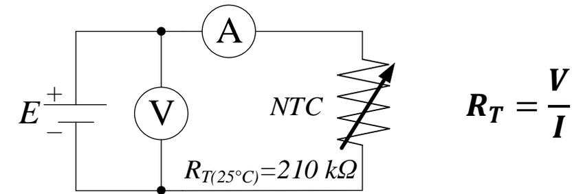
Signal conditioning circuit for typical temperature measurement by exploiting a DC supply voltage
