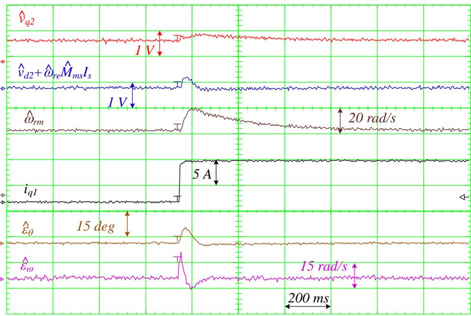
Torque transient from no load to rated torque at  $\omega_{rm} = 50 \text{ rad/s}$ , with the switch SW set to 0, that is to say with the MVPT deactivated
