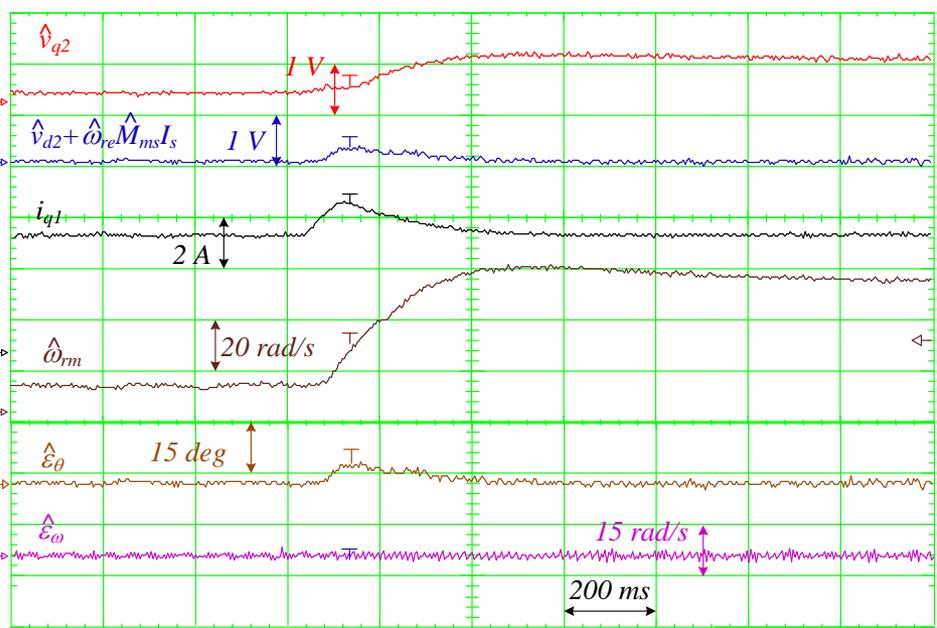
Speed transient from  $\omega_{rm} = 10 \text{ rad/s}$  to  $\omega_{rm} = 50 \text{ rad/s}$  at rated torque, with the switch SW set to 0, MVPT deactivated
