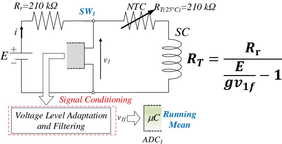
Signal conditioning circuit for proposed temperature measurement with a DC supply of the series connection of the thermistor and SC
