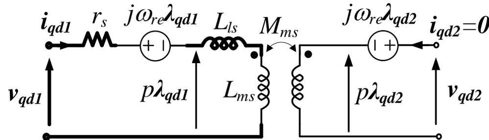
Equivalent circuit of the SMPMSM in the  $qd0$  synchronous reference frame.
