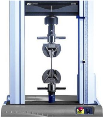
Equipment for tensile test
