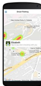
A mechanism based on BLE Advertising is adopted to detect passengers. Furthermore, once the user starts driving, the application starts retrieving GPS position at regular intervals sending them to a remote server which builds a path joining all user GPS points received from the application until the destination is reached. These paths are compared through an algorithm that checks their similarity in order to estimate the number of parking slots still available.
